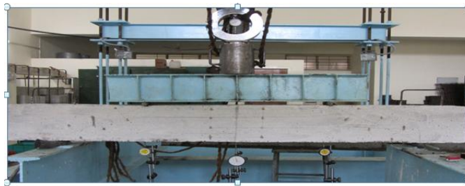
Figure 1: Test Setup of a Typical Beam
